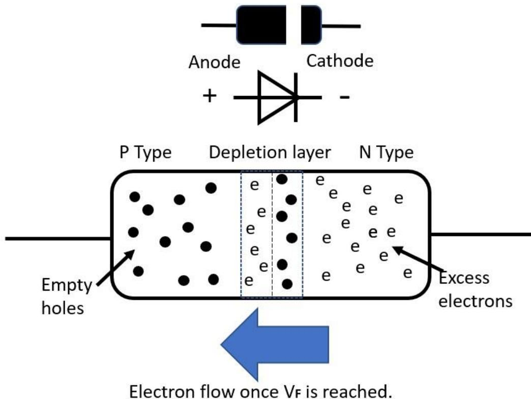
Figure 2: N and P type junction.
