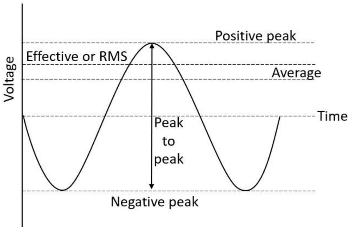
Figure 5: RMS diagram.
