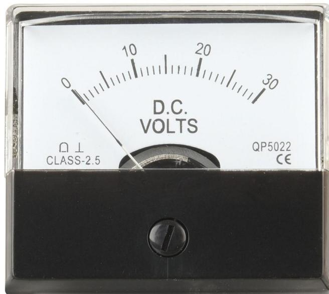
Figure 1: Moving Coil Meter (MCM).
