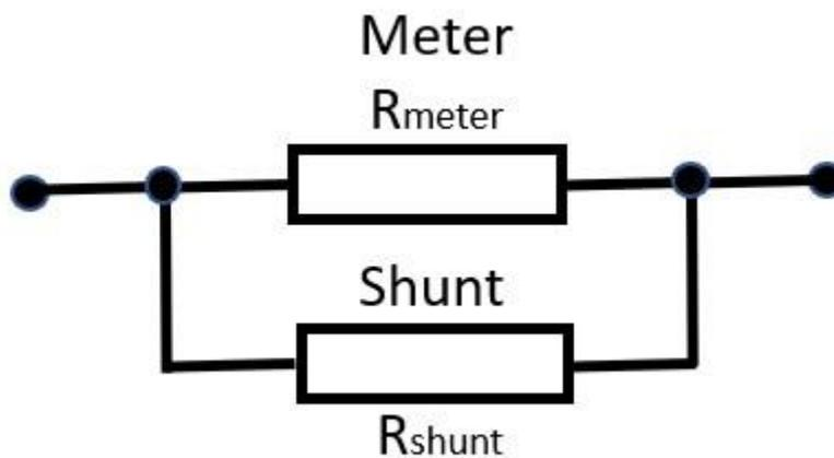
Figure 4: Shunt circuit calculations.
