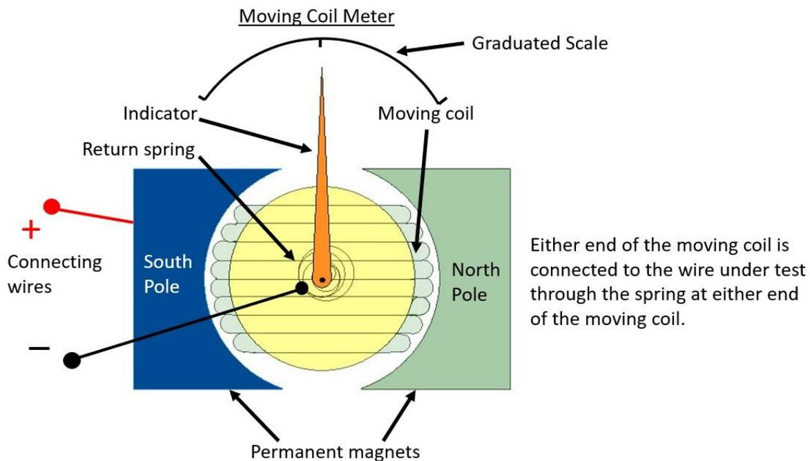
Figure 2: Moving Coil Meter (MCM) Diagram.
