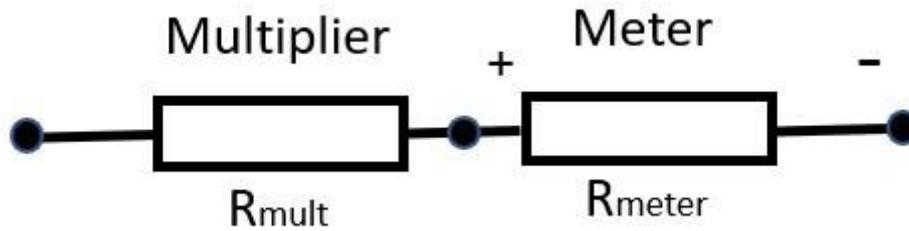
Figure 3: Multiplier circuit calculations.
