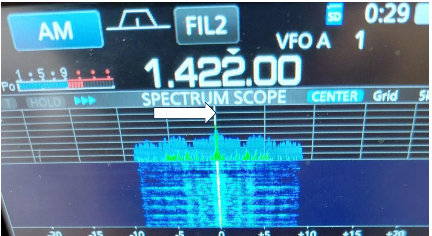
A double-sided AM signal with the centre carrier at 1.422 MHz.
