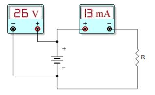
4. What is the resistor value in the given circuit?
