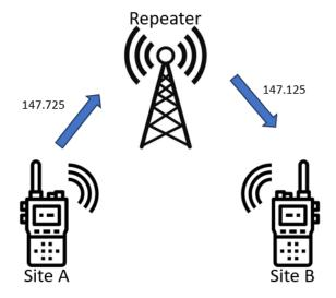
When both radios stop transmitting, they revert to the listening frequency of 147.125MHz.
