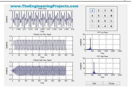
**Example:** You wish to transmit the number 6 over the radio. When you press the number 6 button, the two tones 770 Hz and 1477 Hz are sent. The receiver has a matrix of filters to analyse the tones and confirm the number as 6.
