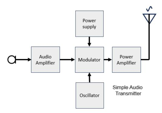
The information to be transmitted is modulated with an oscillator at the carrier frequency. This modulated signal is amplified and sent the antenna.
