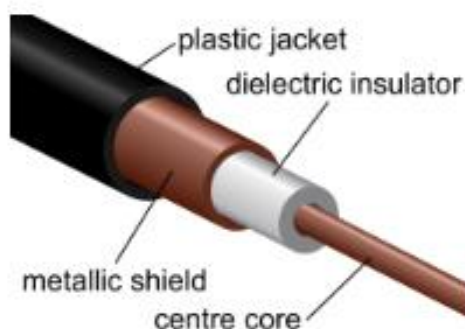
Cutaway image of a shielded cable. Image credit: Tkgd2007
